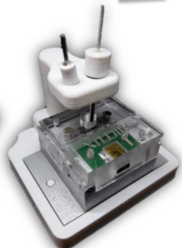
Platform with external Reference & Auxiliary Electrodes
