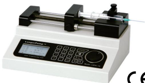
**LSP01-3A** is a single-channel syringe pump which only have infusion mode. These pumps are very easy to operate including a LCD display with rotary coded switch and a simple membrane keypad.
